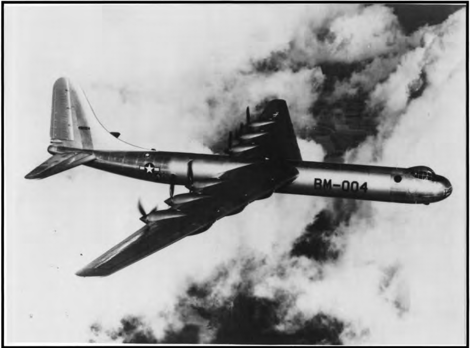
Designed late in WWII, the B-36A bomber patrolled the Cold War-era skies in the days before jets. Designed to "...carry 10,000 pounds of bombs for 10,000 miles" this behemoth was powered by six 28-cylinder engines and carried a 14-man crew. Bob Van Tuyl designed part of the 230-foot-span wings [National Air & Space Museum].
